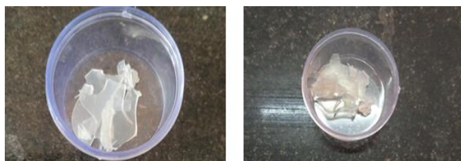
Fig. 5 The starch based polyester synthesized from (a) potato and (b) sweet potato
